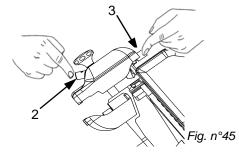
*N.B.*: Do not carry on the deburring operation for more than 3/4 sec. to avoid the damaging bending of the blade edge.
