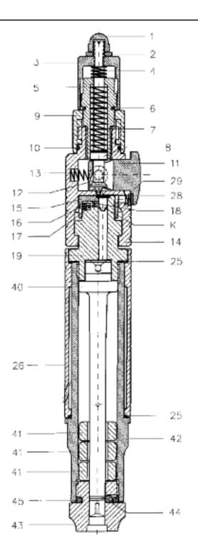
Mechanical cartridge ejector, extended bolt (see appendix 10.1.5)
